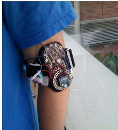
Fig. 1. Initial prototype of the health-monitoring system
