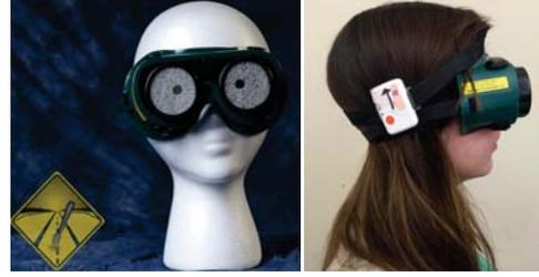
Fig. 5 Glaucoma simulator, from Fork-in-the-Road<sup>®</sup> [6] (left); A participant wearing the glaucoma simulator and the Shimmer<sup>®</sup> wearable motion sensor unit (right).
