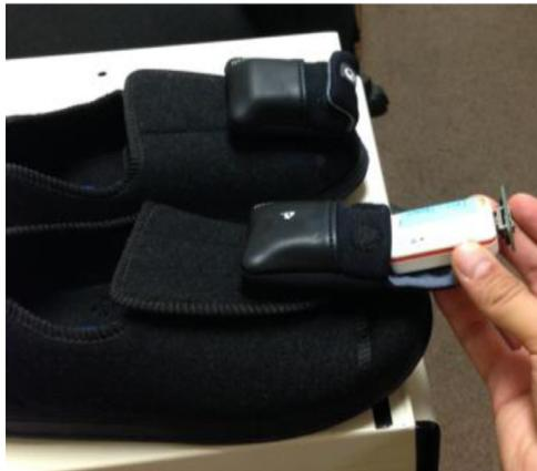
Fig. 2. The sensor-equipped shoes with Shimmer® sensor devices.
