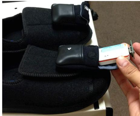
Fig. 1 The sensor-equipped shoes with Shimmer® sensor devices
