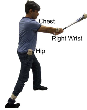
Fig. 1. Experimental subject with three sensor nodes placed on “hip,” “chest,” and “wrist” to capture “hip rotation,” “shoulder rotation,” and “arm extension.”
