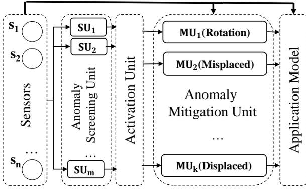
Figure 2: Energy-efficient uncertainty management framework with the anomaly screening unit (ASU).
