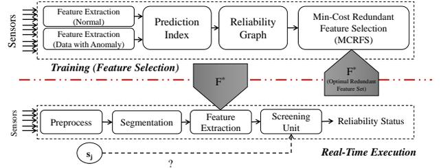
Figure 3: The process of developing the anomaly screening module.
