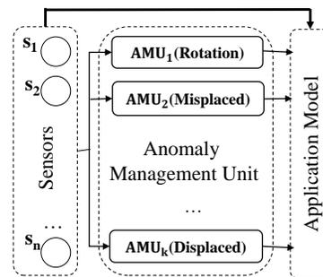
Figure 1: Current uncertainty management approaches in networked wearables. This approach combines detection and mitigation of anomalies into one module called anomaly management unit (AMU).
